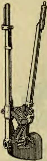
FIG. 455.—Characteristic side lever control. The two levers have distinctive constructions, the brake lever having an external latch mechanism and the transmission lever being provided with a press button at the top of the handle and connection running through same to the latch.
